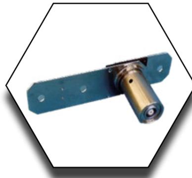
**TERM** ribbon type termination resistors are used when it is difficult to obtain correct impulse shape while testing transformer windings of low impedances. These resistors help to increase the impedance of the test object and are usually utilized together with additional parallel resistors and the Glaninger Circuit.
