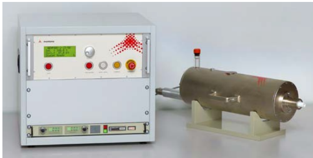
Coaxial pulse generator – 80 kV/m – rise time 1 ns
