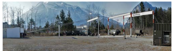
NEMP test system - h = 9.1 m, V = 800 kV
