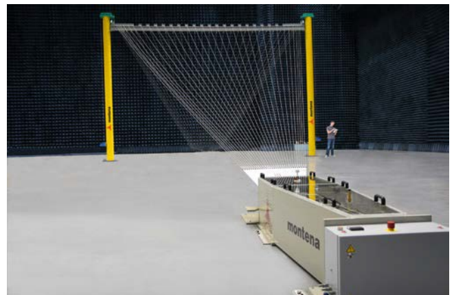
Mobile NEMP test system - h = 7.2 m, V = 520 kV
