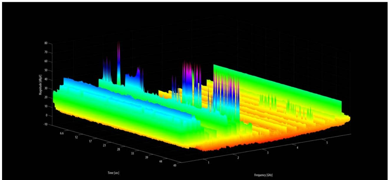
Real-time measurement 30 MHz - 6 GHz, Bluetooth inquiry process at 2,4 GHz.
