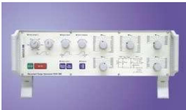
All impulse circuit components may be adjusted in steps. The impulse shape can thus be fine-tuned within a wide range. Additional capacitors and resistors can be connected externally to permit operation with larger impulse capacitances and other resistance values. The peak value of the impulse voltage is stabilized and continuously adjustable. The voltage impulse may be chopped internally within broad limits.
